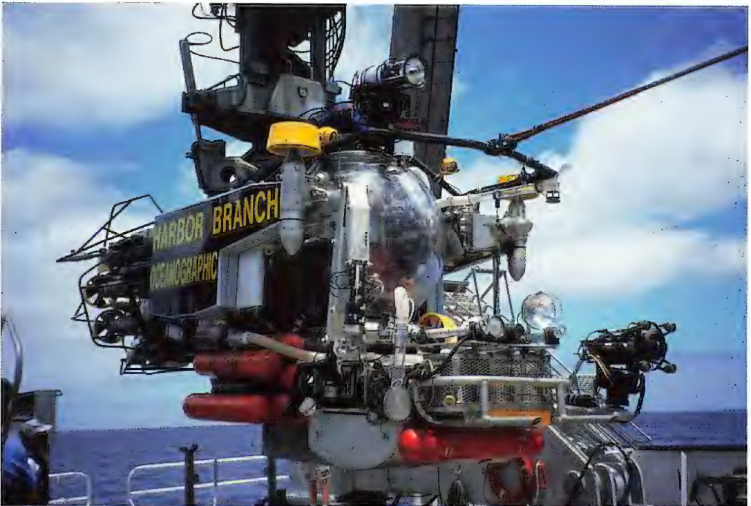
FIGURE 3. Johnson-Sea-Link submersible on deck of R/V Seward Johnson . The specimen collecting equipment, viewed in a counter clockwise direction is as follows: video camera (lower right); plankton capture funnel (upper right); articulated claw (left side); vacuum hose and rotenone dispenser (small clear tubing attached to hose) (lower left); storage basket (lower center). A laser-aimed still camera resides atop the storage basket. Not visible is the carousel of specimen-holding aquaria. Photo credit J. McCosker.
